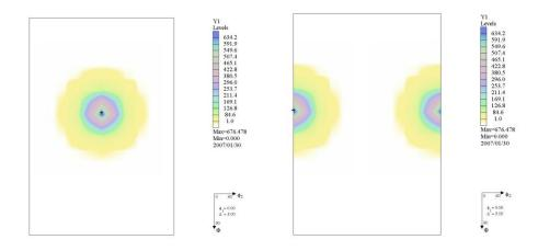
Example below shows sections of ODFs with great participation of component  $\{-124\}<210>$  which were input to LaboTex in bad convention. For both hexagonal conventions the marks indicate position of orientation belong to $\{-124\}<210>$  component when maximum of ODF are moved to incorrect position (section of ODF in the first convention is shown on the figure from left and section of ODF in the second convention is shown on the figure from right).
