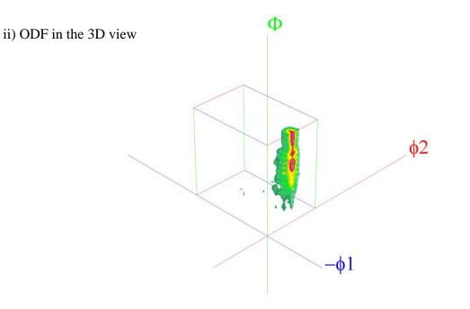
Example of ODF of sample with strong  $\{112\}<1-10>$  texture component in the second hexagonal convention (component  $\{112\}<1-10>$  in Euler angles (0,58,0)): i) ODF projection  $\phi_2$ ;
