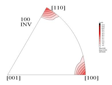
Below you can see that when you choose Y (i.e. (010) or TD) direction for inverse pole figure then the planes type  $\{010\}$  (the plane (010) is marked on the red in the figure) is perpendicular to this direction for orientation  $\{001\}<100>$ .
