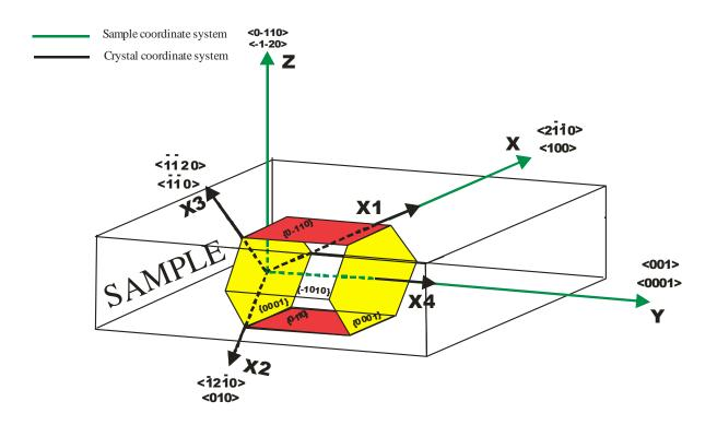
the basal planes are perpendicular to TD (Y) direction hence in this case the inverse pole figure calculated for this direction shows maximum for <001> direction:
