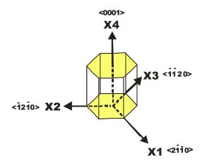
Plane in Miller-Bravais Notation: {HKTL} Direction in Miller-Bravais Notation <UVTW> T=-(H+K) (redundant information) <UVTW> direction in Miller-Bravais Notation is perpendicular to {UVTW} plane (similar as in Miller Notation in cubic system).
