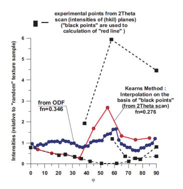
The radial Kearn's texture parameter ( $f_r$ ) is usually greater than 0.5 for Zircaloy nuclear fuel clad tubing. (See also: Van Swam, L. F. P. et al; "*Relationship Between Contractible Strain Ratio R and Texture in Zirconium Alloy Tubing*"; Metallurgical Transactions A, Volume 10A, pages 483-487. (1979)).
