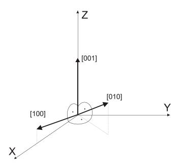
Crystal and sample coordinate systems. General LaboTex Axes and Angles Convention (example for righ- handed coordinate systems)
