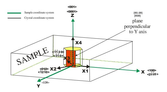
The perpendicular direction  $\langle 120 \rangle$  will represent this plane on the inverse pole figure. Because direction  $\langle 120 \rangle$  doesn't belong to the unit triangle (main, fundamental area) the equivalent direction  $\langle 210 \rangle$  from unit triangle is choosen:
