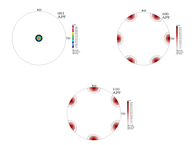
In case of inverse pole figures for RD and TD directions (XYZ=<100> and XYZ=<010>) we can observe the different positions of maximum for orientation  $\{001\}<100>$ . The plane perpendicular to X axis is  $\{2-1-10\}$ :
