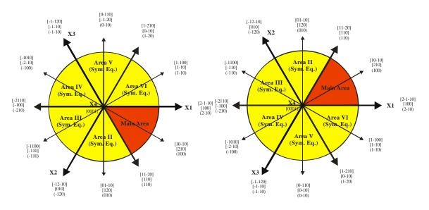
Below you can see examples of complete (full) and partial inverse pole figures for hexagonal crystal system (example calculated for strong component {-124}<210>, c/a=1.6):
