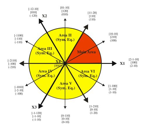
Below you can see the inverse pole figure for TD direction with maximum for direction <210>(<10-10>) determined by the planes: {100} or {10-10}.
