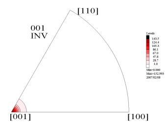
Pole figures (001), (100) and (110) for orientation  $\{001\}<100>$  show position of basal planes  $\{0001\}$ , first order prism planes  $\{10-10\}$  and second order prism planes  $\{2-1-10\}$ :
