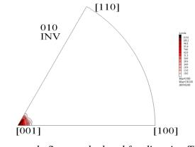
Inverse pole figure calculated for direction TD (Model of component {0-10}<100>, FWHM 10 degrees)
