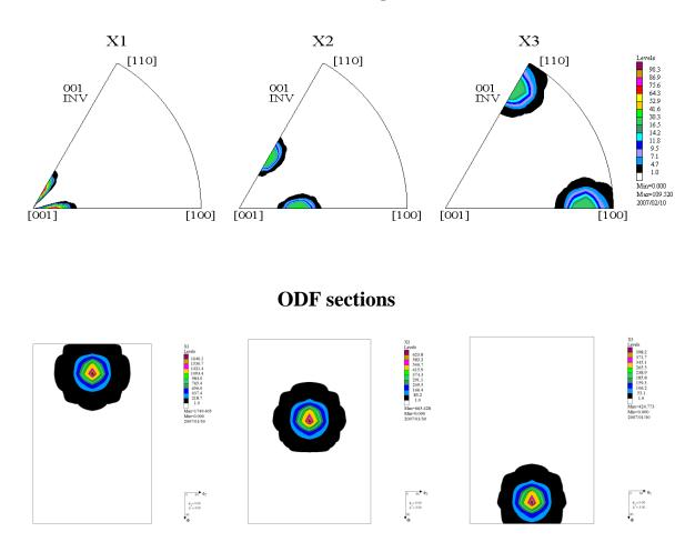
In hexagonal crystal system Euler angles for orientation  $\{-124\}<210>$  depend on cell parametres, hence when LaboTex shows poles for orientation given by Euler angles according to first pole figure i.e. $\{0,14,330\}$  the others shows marks not in maxims (Euler angles for orientation  $\{-124\}<210>$  for second and third case of c/a are equal respectively  $\{0,39,330\}$  and  $\{0,79,330\}$ ).
